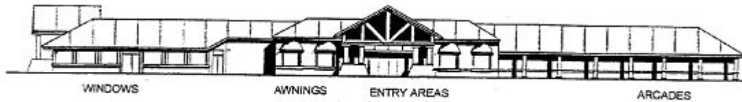
Animating features such as these must total 60% of total facade length for any facade abutting a public street
